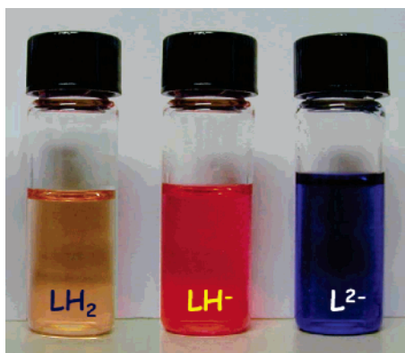
FIGURE 1. Color changes observed on addition of [\text{Bu}_4\text{N}]\text{F} to a DMSO solution of receptor 1 ( = \text{LH}_2 ). Left to right: no addition (dominant species: \text{LH}_2 ); plus 5 equiv of [\text{Bu}_4\text{N}]\text{F} (dominant species: \text{LH}^- ); plus 40 equiv of [\text{Bu}_4\text{N}]\text{F} (dominant species: \text{L}^{2-} ).
